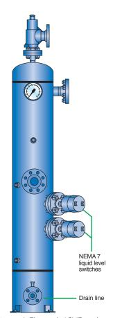
Figure 4: Flanged, ASME code liquid trap with liquid-level switches, manual drain, and stainless steel demister pad.
