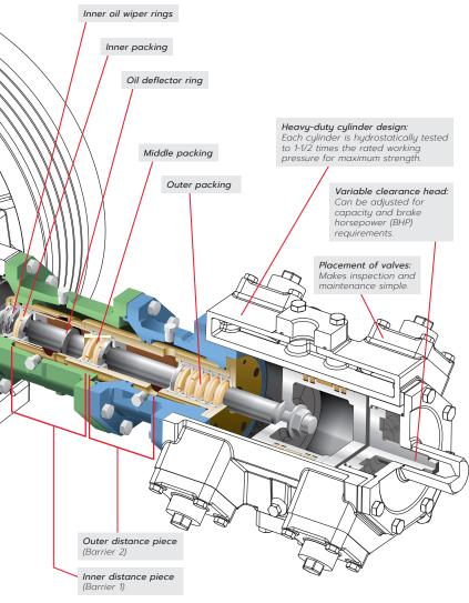
corrosive or toxic applications where leakage containment and non-contamination of the gas stream are critical.
