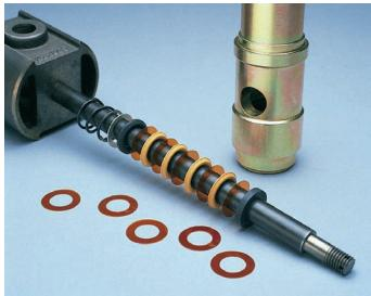
Crosshead guide, piston rod, packing barrel, K-ring spacers, and packing set.
