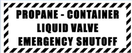
V-127 Red on White Vinyl 30" x 12" with required 2" letters for Emergency Remote Shutdown Station
